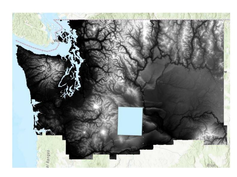
3. Then it will use the polygon vector layer to make a new DEM with the target domain area clipped out of the original parent DEM.
