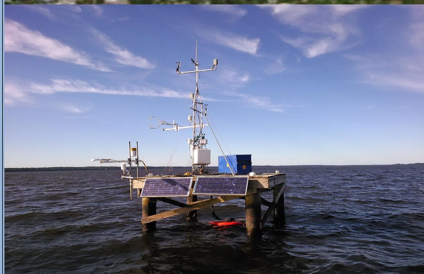
Figure 2: The RBR eddy covariance flux tower located roughly 2 km from reservoir shore
