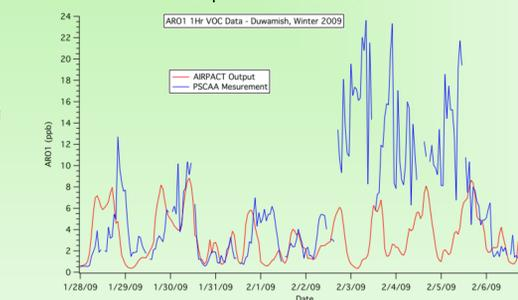
**Figure 7:** Observed and predicted concentrations for VOCs lumped into the SAPRC-99 group ARO1 during winter. Lows are predicted more successfully, but peaks are often missed.
