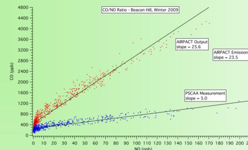
**Figure 5:** Observed and predicted CO/NO ratio at Beacon Hill during winter. Observed values are much lower than predicted values, and there's a significant gap between the slope of both data sets.
