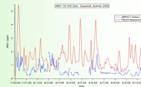
**Figure 8:** Observed and predicted concentrations for VOCs lumped into the SAPRC-99 group ARO1 during summer. Predicted values are consistently higher than observed values throughout the period.
