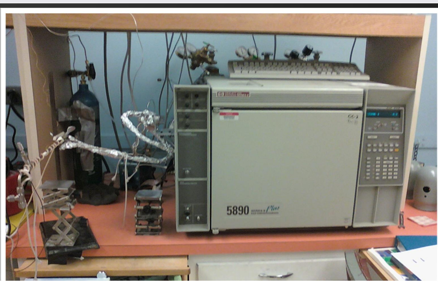
Figure 2. GC/FID used for the analysis of non-methane hydrocarbons from MBO samples
